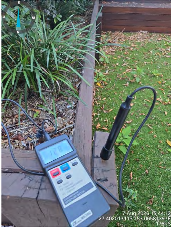
P11 - Moisture testing at a planter corner with garden bed immediately adjacent.
